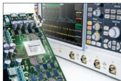
▲ Fig. 3 All signal processing takes place in the recording trigger control ASIC.
