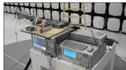
▲ Fig. 6 Down-conversion system, DSA, AWG and PSG.
